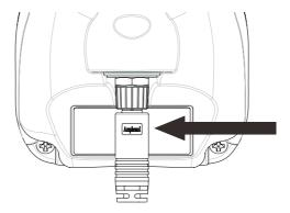
4) The transmitter is designed to accept any off-the-shelf Ni-MH rechargeable batteries. Depending on the battery capacity the average charging time is approximately 1.5 hours from completely drained to fully charged. Constant red on the LED represents charging in progress, constant green represents batteries fully charged, and LED off represents no batteries detected. Please do not use any rechargeable lithium ion batteries as it will damage both the transmitter and the charging station.
