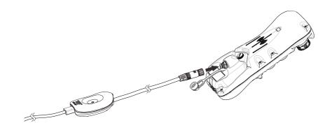
3) Make sure the marking on the charging plug (see below) is facing the top side when connecting.
